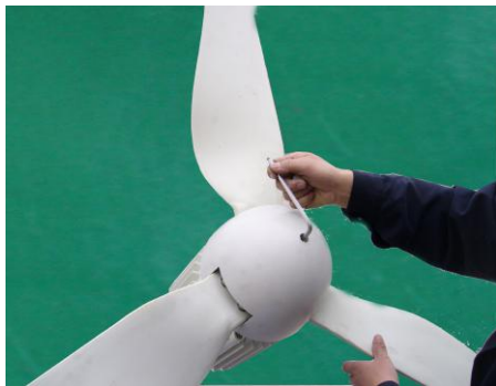
3、 TIGHTEN THE FRONT COVER BY FRONT COVER BOLT
