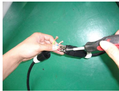
2、 PULL OUT THE CABLE COVER AND CONECT THE CABLE'S THREE FAHSE WIRE WITH WIND TURBINE THREE PHASE WIRE
