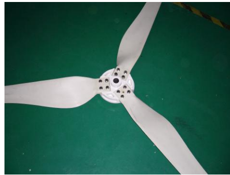
4、 ASSEMBLE THE BLADES WITH BLADE NUTS
