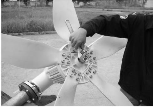
(9) Mounting the hub with blades onto the motor shaft.
