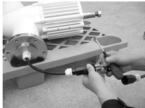
(6) Screwing out one terminal of cable cover and connect the cables three-phase wire with wind turbine three-phase wire.
