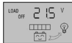
At this interface, press the button  $\text{enter}$  for long ( $>5$ seconds) , the number starts to flicker, and it means the controller enters into the interface of setting the protection voltage.
