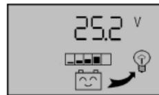
At this interface, press the button  $\text{enter}$  for long ( $>5$ seconds), the number starts to flicker, and it means the controller enters into the interface of setting the recovery voltage.
