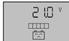
and the load loop disconnects. Use the solar panels or charger to charge for the battery .When battery voltage recovers to the protection voltage, the controller will recover to supply power for load and enter into the working state.
